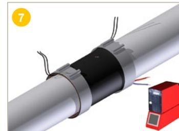
⚠ **Allow** the muff to cool before electrowelding. After shrinking and cooling to ambient temperature, **fit** the tightening straps on the heat-shrinkable muff.
